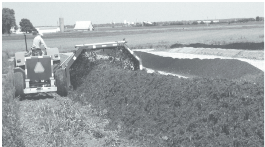
Figure 44-7. Mechanical turner used in composting solid manure.
