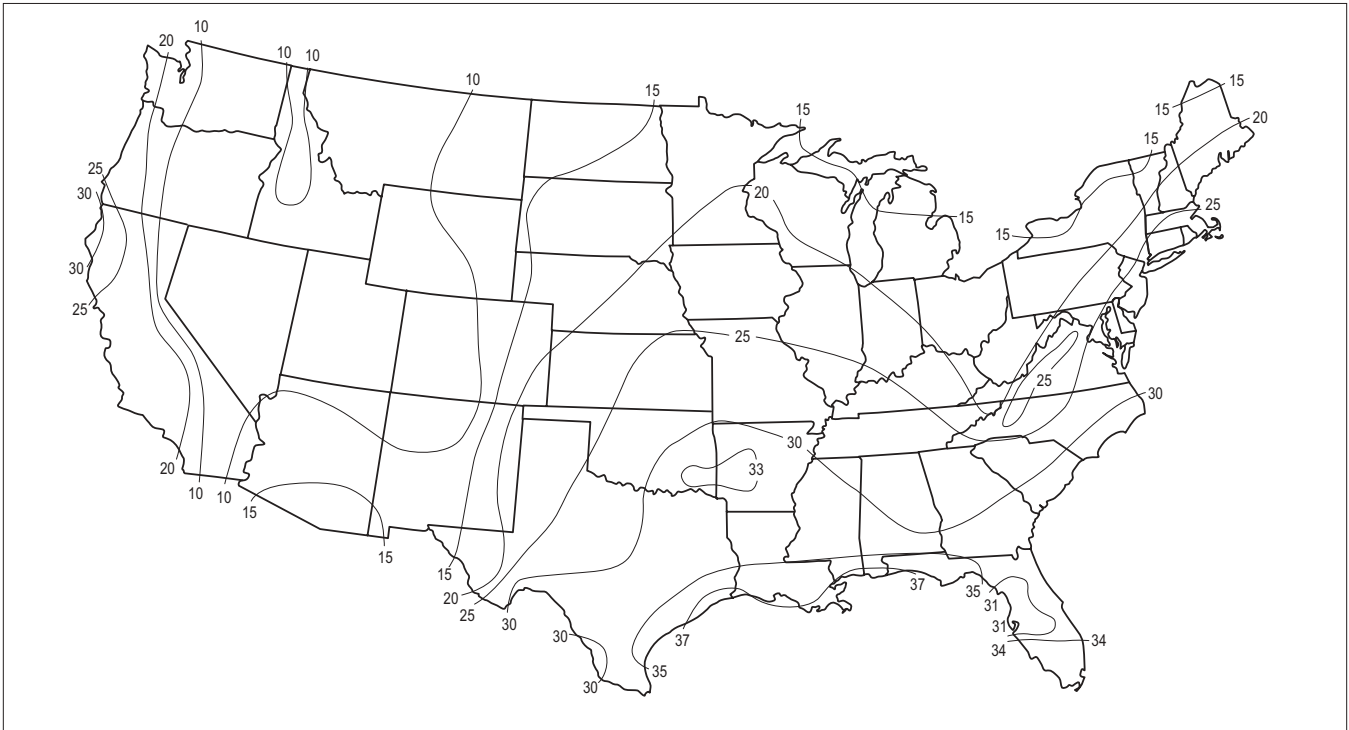
Figure 21B-1. Annual runoff from unsurfaced feedlots (CN-90) as percent of mean annual precipitation.
