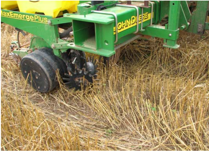
Trash wipers need to clean residue, but disturb the soil as little as possible to conserve moisture.
