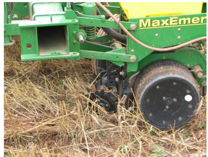
Finding the best combination of down pressure and seeding depth may require some experimentation with planter adjust-
